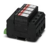
Lightning/surge protective device for 2-pos. isolated 1000 V DC voltage systems, for DIN rail mounting, 4-pos. base element with remote indication contact, four plug-in temperature-monitored protective elements, status message on each plug.
