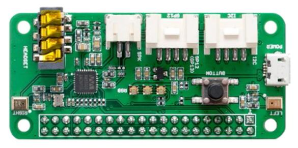
ReSpeaker 2-Mics Pi HAT is a dual-microphone expansion board for Raspberry Pi designed for AI and voice applications. This means that you can build a more powerful and flexible voice product that integrates Amazon Alexa Voice Service, Google Assistant, and so on.
