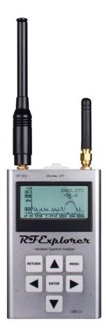
RF Explorer is a handheld digital spectrum analyser, a very affordable tool for work in all ISM popular frequency bands. It is based on a highly integrated frequency synthesizer which offers high performance, compact size, low consumption and low cost.
