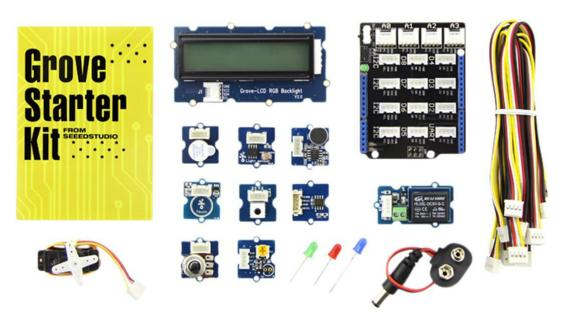
Grove is a modular electronic platform for quick prototyping. Every module has one function, such as touch sensing, creating audio effect and so on. Just plug the modules you need to the base shield, then you are ready to test your idea buds.
