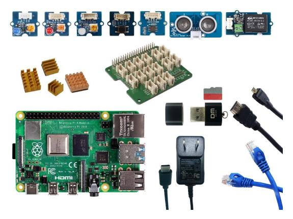
The Grove Base Kit for Raspberry Pi is one of the best kits for beginners to get started with Raspberry Pi. No troublesome soldering and no complicated wiring. You can focus on learning Raspberry Pi. This kit includes a Grove Base Hat for Raspberry Pi and 7 Grove. All you need to do is follow the demo and plug the module into the Grove Base Hat, truly plug and play.
