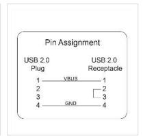
The USB Type A Port Blocker blocks the data lanes of the used USB port and thus protects your end device from unwanted access or malware - nothing but power is transmitted. The solution is especially useful in foreign environments where USB sockets can be manipulated or hijacked comparatively easily, such as in hotels, or anchorage points like airports or train stations.
