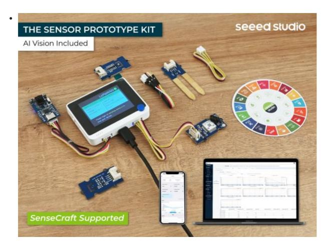
SenseCAP K1100 is an open-source prototype kit designed to incentivize the co-creation of IoT sensors to tackle real-world challenges. It is compatible with easy-to-start programming platforms like Arduino for customized coding. In addition, users can also train the Wio Terminal TinyML models using in-builds and Grove sensors.
