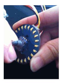
**Note:** It is able to generate another signal when it's being pressed down. However due to the limitation of the number of Grove signal cable, the module is made without output of this signal.
