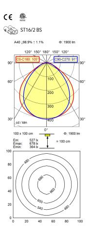
light source work equipment connected load power consumption luminous flux luminous efficiency light distribution direct ratio beam angle colour temperature colour temperatur color rendering index (CRI) chromaticity tolerance LED glare control luminance (L65) unified glare rating (4H 8H) system of protection class of protection technology operation housing weight (net) mains lead fastening dimension light output side part special features
