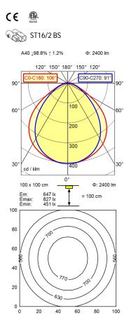
light source LED work equipment without connected load 22-26 V, DC env. 31.5 W power consumption luminous flux approx. 2.400 lm luminous efficiency approx. 75 lm/W light distribution direct direct ratio approx. 99 % 100° beam angle colour temperature neutral white
