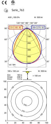
light source LED without work equipment connected load 20-28V, DC env. 5 W power consumption luminous flux approx. 500 lm luminous efficiency approx. 100 lm/W light distribution direct 80°/90° beam angle
