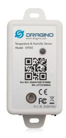
The Dragino LHT65 Temperature & Humidity sensor is a Long Range LoRaWAN Sensor. It includes a **built-in SHT20 Temperature & Humidity sensor** and has an external sensor connector to connect to external sensors such as **Temperature Sensor, Soil Moisture Sensor, Tilting Sensor** etc.
