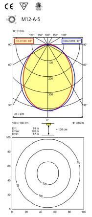
light sourceLEDwork equipmentwithoutconnected load22-26 V, DCpower consumptionenv. 3 Wluminous fluxapprox. 315 lmluminous efficiencyapprox. 105 lm/W
