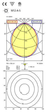
light sourceLEDwork equipmentwithoutconnected load22-26 V, DCpower consumptionenv. 6 Wluminous fluxapprox. 630 lmluminous efficiencyapprox. 105 lm/W
