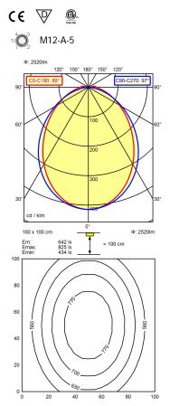
light sourceLEDwork equipmentwithoutconnected load22-26 V, DCpower consumptionenv. 24 Wluminous fluxapprox. 2.520 lmluminous efficiencyapprox. 105 lm/W
