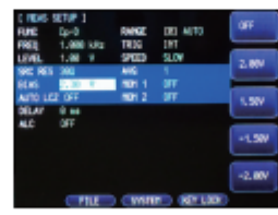
Internal Bias (±2.5V Adjustable) Ideal for Capacitive Components' Characteristic Tests
