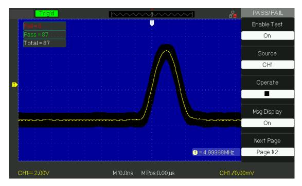
With easy to generate user-defined test templates, the RSDS1000DL+/CML+ compares the current measured trace to the template mask trace making it suitable for long-term signal monitoring or automated production line testing.
