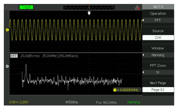
RSDS1000DL+/CML+ provides 5 kinds of math operation: +, -, \*, /, FFT, supporting channel waveform and FFT waveform in either split display windows or both signals appearing on the full screen.
