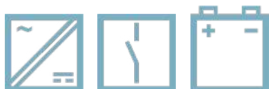
Power supply UPS module Energy storage devices
