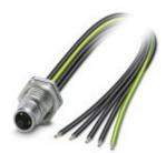
Flush-type connector, Power, 5-position, Plug, M12, K - Power, Rear mounting, M16 x 1.5, Individual wires, cable length: 0.2 m
