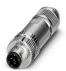
Bus system connector, PROFIBUS DP (12 Mbps), 2-position, shielded, Plug straight M12, B-coded, Push-in connection, knurl material: Zinc die-cast, nickel-plated, external cable diameter 4 mm ... 8 mm
