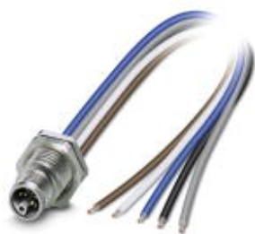
Flush-type connector, Power, 5-position, Plug, M12, L - Power, Rear mounting, M16 x 1.5, Individual wires, cable length: 0.2 m
