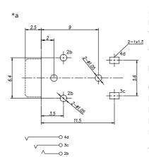
\*a printed circuit board layout, solder side view
