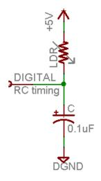
In this case, our 'bucket' is a 0.1uF ceramic capacitor. You can change the capacitor nearly any way you want but the timing values will also change. 0.1uF seems to be an OK place to start for these photocells. If you want to measure brighter ranges, use a 1uF capacitor. If you want to measure darker ranges, go down to 0.01uF.
