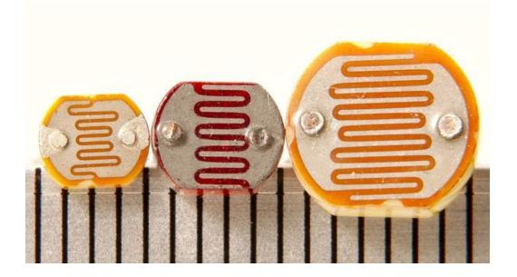
For most light-sentsitive applications like "is it light or dark out", "is there something in front of the sensor (that would block light)", "is there something interrupting a laser beam" (break-beam sensors), or "which of multiple sensors has the most light hitting it", photocells can be a good choice!
