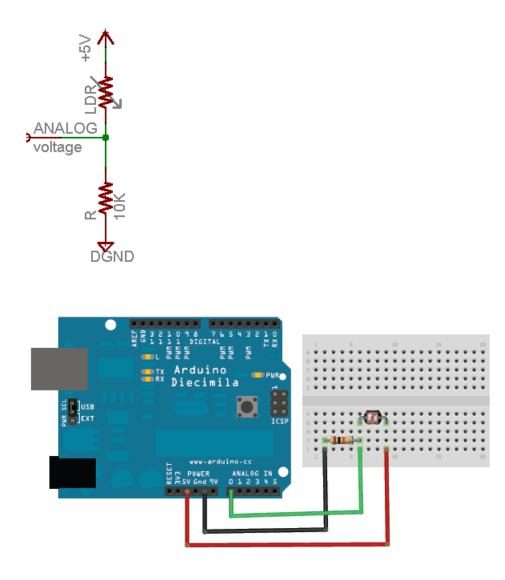
For this example I'm showing it with a 5V supply but note that you can use this with a 3.3v supply just as easily. In this configuration the analog voltage reading ranges from 0V (ground) to about 5V (or about the same as the power supply voltage).
