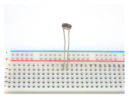
Photocells are pretty hardy, you can easily solder to them, clip the leads, plug them into breadboards, use alligator clips, etc. The only care you should take is to avoid bending the leads right at the epoxied sensor, as they could break off if flexed too often.
