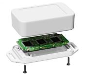
A 1.6 mm thick PCB can be clamped directly between the enclosure parts and optionally hot melted and clenched via two pins.
