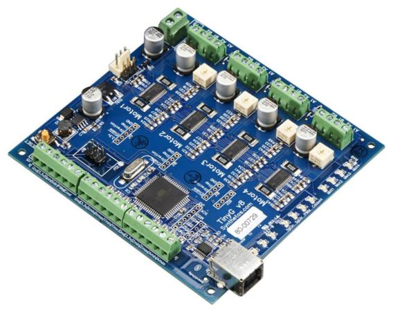
The TinyG project is a high performance, USB based CNC 6-axis controller that supports XYZ linear and ABC rotary axes with 4 motor outputs. It is designed for small CNC applications and other applications that require highly controllable motion control. TinyG is meant to be a complete embedded solution for small or medium motor control.
