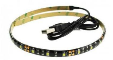
Our 5V LED Single colour tape uses long life super bring LEDs and features very low power consumption of just 4.8watts per metre for the 60 LEDs per metre. Our range of LED Strip lighting is supplied on a flexible printed circuit board (PCB) which is white / black in colour had has a 3M sticky tape backing making installation extremely easy. Just peel off the backing cover and stick down to any flat clean surface
