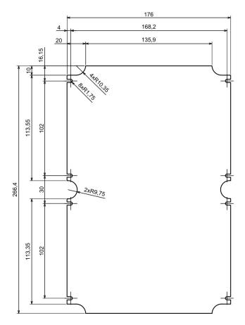
All dimensions are given within +/-0,5mm tolerance
