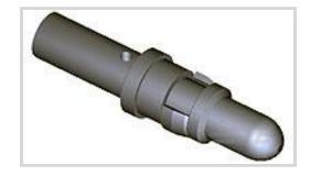
Contact Type: Pin D-Sub Contact Size: 8 Contact Base Material: Copper Alloy Contact Mating Area Plating Material: Gold Termination Method to Wire & Cable: Crimp
