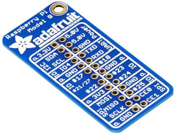
This board makes it easy to see if you're connecting your wires correctly to the Raspberry Pi GPIO. Design licensed from Low Voltage Labs' Pi GPIO Reference Board, with some changes – including grouping the pins into categories like I2C, IO, UART, SPI, and power.
