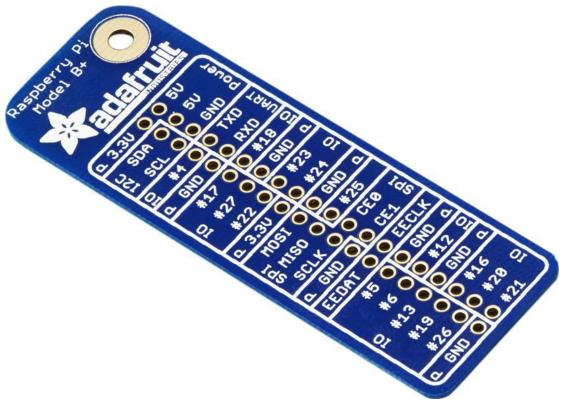
This board makes it easy to see if you're connecting your wires correctly to the Raspberry Pi GPIO. Design licensed from Low Voltage Labs' Pi GPIO Reference Board, with some changes – including grouping the pins into categories like I2C, IO, UART, SPI, and power.
