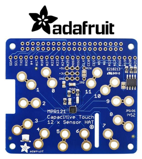
This touchable add-on HAT for Raspberry Pi will inspire your next interactive project with 12 capacitive touch sensors. Capacitive touch sensing works by detecting when a person has touched one of the sensor electrodes. Capacitive touch sensing used for touch-reactive tablets and phones, as well as control panels for appliances. This HAT allows you to create electronics that can react to human touch, with up to 12 individual sensors.
