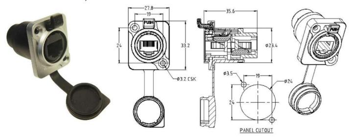
A metal frame Cat5e RJ45 feedthrough socket with IP65 rating. The compatible XLR style plug carrier
