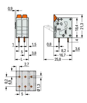
$L = (pole no. - 1) \times pin spacing + 7.4 mm$
