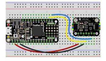
Board 3V to sensor VIN Board GND to sensor GND Board SCL to sensor SCK Board SDA to sensor SDI
