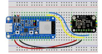
Board 3V to sensor VIN (red wire on STEMMA QT) Board GND to sensor GND (black wire on STEMMA QT) Board SCL to sensor SCL (yellow wire on STEMMA QT) Board SDA to sensor SDA (blue wire on STEMMA QT)
