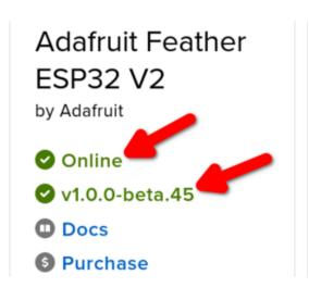
On the device page, quickly check that you're running the latest version of the WipperSnapper firmware.
