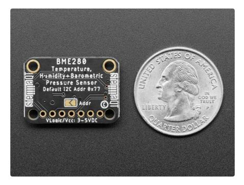
Nice sensor right? So we made it easy for you to get right into your next project. The surface-mount sensor is soldered onto a PCB and comes with a 3.3V regulator and level shifting so you can use it with a 3V or 5V logic microcontroller without worry.
