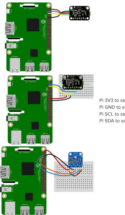
Pi 3V3 to sensor VIN Pi GND to sensor GND Pi SCL to sensor SCK Pi SDA to sensor SDI
