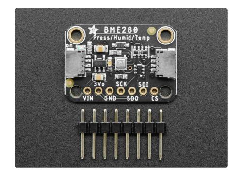
The BME280 is the next-generation of sensors from Bosch, and is the upgrade to the BMP085/BMP180/BMP183 - with a low altitude noise of 0.25m and the same fast conversion time. It has the same specifications, but can use either I2C or SPI. For simple easy wiring, go with I2C. If you want to connect a bunch of sensors without worrying about I2C address collisions, go with SPI.
