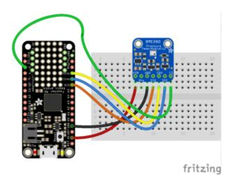
Board 3V to sensor VIN Board GND to sensor GND Board SCK to sensor SCK Board MOSI to sensor SDI Board MISO to sensor SDO Board D5 to sensor CS (or use any other free digital I/O pin)
