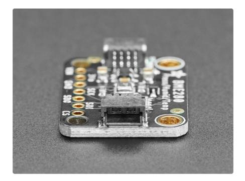
The breakout is made in the <u>STEMMA QT form factor</u> (https://adafru.it/LBQ), making them easy to interface with. The <u>STEMMA QT connectors</u> (https://adafru.it/JqB) on either side are compatible with the <u>SparkFun Qwiic</u> (https://adafru.it/Fpw) I2C connectors. This allows you to make solderless connections between your development board and the BME280 or to chain it with a wide range of other sensors and accessories using a compatible cable (https://adafru.it/JnB).
