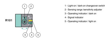
To unlock the adjustment functions turn the sensing range adjuster for more than 180 degrees.
