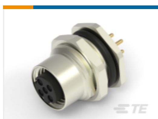
TE Part #T4141516041-000 M12,REAR MOUNT,FEMALE,D,4P, M16,POTTING
