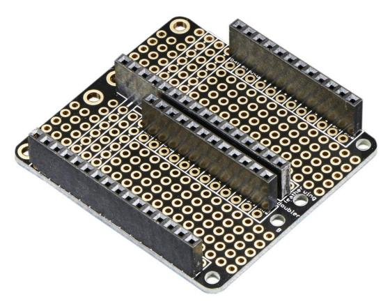
This is the FeatherWing Doubler – a prototyping add-on and more for all Feather boards. This is similar to the FeatherWing Proto except there are two! The magic of the Doubler comes when stacking a Feather and another board on top of the Doubler so you can work with both boards simultaneously side-by-side.
