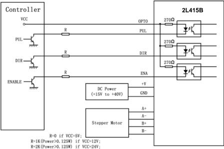
R must be connected to control signal terminal.
