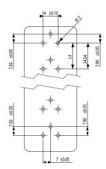
Drilling diagram for PCB terminals: All bussed [mm]
