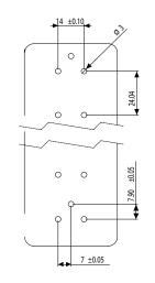
Drilling diagram for PCB terminals: L/N individual and PE bussed [mm]
