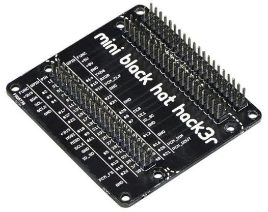
A breakout from Pimoroni that lets you access all of the GPIO pins while also running a HAT or pHAT on your Raspberry Pi Model Zero, 3, 2, A+, or B+ (any Pi with a 2x20 connector). The Pimoroni Mini Black HAT Hack3r is ideal for debugging your (p)HAT projects or combining a (p)HAT with other circuits.
