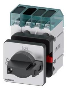
Load disconnector 3LD3, lu 16 A Main switch 3-pole + N Rated operating capacity at AC-23 A at 400V 7.5kW Front plate mounting Basic switch with Central hole mounting 22.5mm Toggle drive black 48x48 mm
