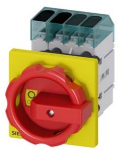
Load disconnector 3LD3, Iu 16 A Main switch 3-pole + N Rated operating capacity at AC-23 A at 400V 7.5kW Front plate mounting Basic switch with Central hole mounting 22.5mm Rotary actuator red / yellow  $66 \times 66$  mm
