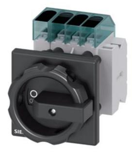
Load disconnector 3LD3, lu 16 A Main switch 3-pole + N Rated operating capacity at AC-23 A at 400V 7.5kW Front plate mounting Basic switch with Central hole mounting 22.5mm Rotating drive black 66 x 66 mm with auxiliary switch 1OE + 1S
