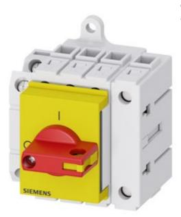
Load disconnector 3LD3, lu 25 A Main switch 3-pole + N Rated operating capacity at AC-23 A at 400V 9.0kW Installation in distribution boards, Basic switch with selector knob red / yellow with auxiliary switch 1OE + 1S
