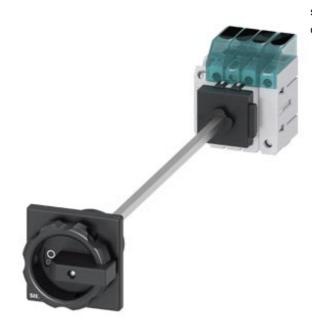
Load disconnector 3LD3, lu 25 A Main switch 3-pole + N Rated operating capacity at AC-23 A at 400V 9.0kW floor mounting Basic switch with door coupling Central hole mounting 22.5mm Rotating drive black  $66 \times 66$  mm with auxiliary switch 10E + 1S
