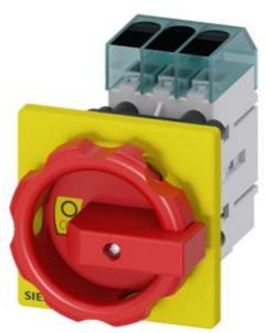
Load disconnector 3LD3, Iu 25 A Main switch 3-pole Rated operating capacity at AC-23 A at 400V 9.0kW Front plate mounting Basic switch with Central hole mounting 22.5mm Toggle drive red / yellow 66x66 mm
