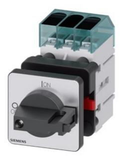
Load disconnector 3LD3, lu 32 A Main switch 3-pole Rated operating capacity for AC-23 A at 400V 11.5kW Front plate mounting Basic switch with Central hole mounting 22.5mm Toggle drive black 48x48 mm
