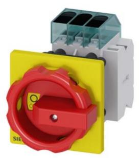
Load disconnector 3LD3, Iu 32 A Main switch 3-pole Rated operating capacity for AC-23 A at 400V 11.5kW Front plate mounting Basic switch with Central hole mounting 22.5mm Rotary actuator red / yellow 66 x 66 mm with auxiliary switch 10E + 1S
