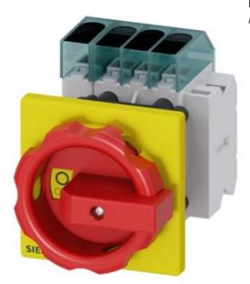
Load disconnector 3LD3, Iu 32 A Main switch 3-pole + N Rated operating capacity for AC-23 A at 400V 11.5kW Front plate mounting Basic switch with Central hole mounting 22.5mm Rotary actuator red / yellow  $66 \times 66$  mm with auxiliary switch 10E + 1S
