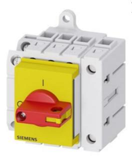
Load disconnector 3LD3, lu 40 A Main switch 3-pole + N Rated operating capacity at AC-23 A at 400 V 15.0 kW Installation in distribution boards, Basic switch with selector knob red / yellow with auxiliary switch 10E + 1S
